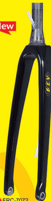
▲ FRC-7072 1-1/8"~1.5" steerer, FM, maxi tire: 700*28C, 12*100mm, internal cable routing
