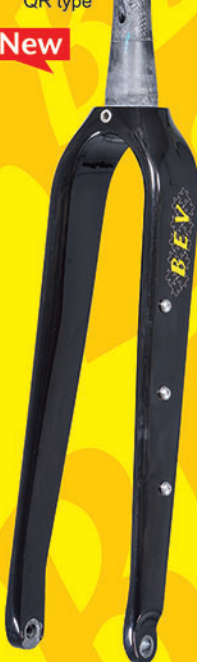
▲ FCC-646-IC 1-1/8"~1.5" steerer, FM, maxi tire: 700*45C, 12*100mm, internal cable routing
