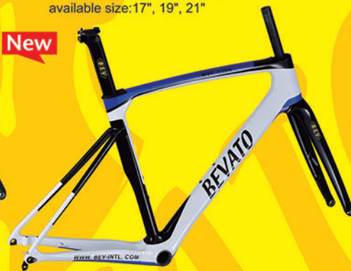
▲ BVC-7108 700c gravel racing, full internal cable routing, including seat post & fork, maxi tire: 700*42C, available size: 46, 48, 51, 53, 56cm
