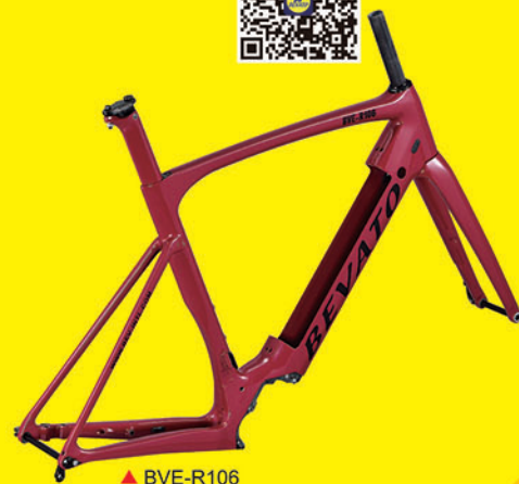
▲ BVE-R106 carbon road E-frame for Bafang M800 (battery Bafang BTF05), maxi tire: 700*32C, available size: 46, 48, 51, 53, 56cm
