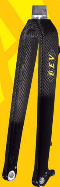
▲ FCC-705-15 1-1/8"~1.5" steerer, PM, maxi tire: 700*45C, 15*100mm
