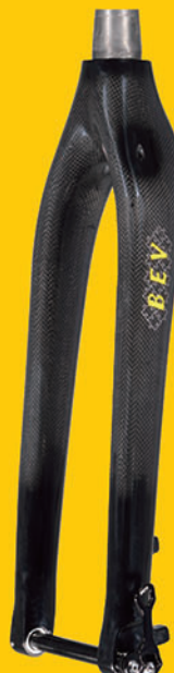
▲ FMC-706 1-1/8"~1.5" steerer, PM, maxi tire: 27.5*2.2" or 29*2.1", 15*100mm, internal cable routing
